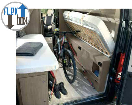
Flexbox: Removable storage modules to adapt how the space is used
