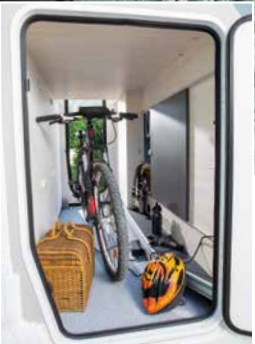
Heated, illuminated garage holds, equipped with stowage hooks, electric plugs 12V/230V and 2 doors
